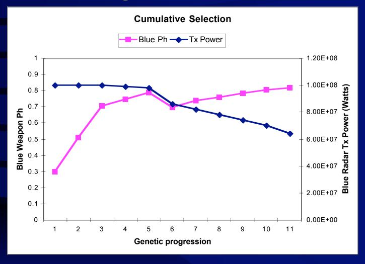
Blue Cost Effectiveness increases as the weapon Ph increases (less weapons needed for same effect) and as radar Tx power diminishes (two reasons: cheaper radar, and reduced "observables.")
