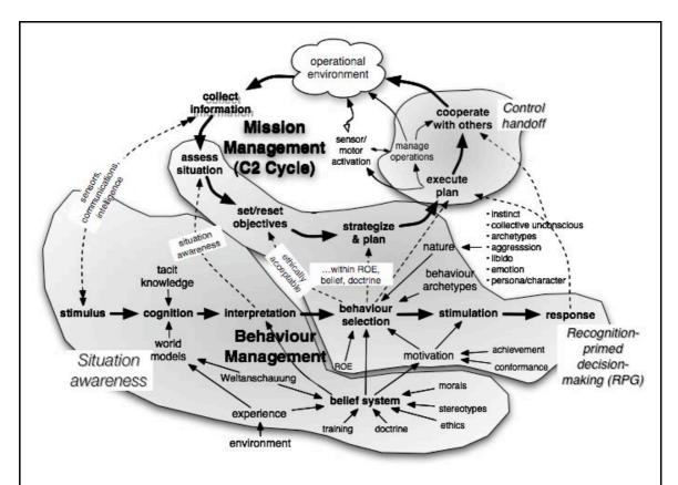
**Figure 11. Developing Functional Architecture**. Figure 5 showed the design reference framework. The figure above shows how three major design subsystems map on to that framework: Situation awareness; Recognition-primed decision-making; and Control handoff – effectively, the management of operations, through sensor/motor activation. In effect, the design study is generating a number of interacting 'cerebral' cortices...
