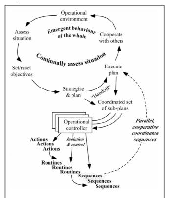
**Figure 8.** Control Handoff. The command loop is continuously busy as situations change. Control of the *execution* of strategies and plans is 'handed-off' to operational controllers, who manage the execution of coordinated sets of sub-plans, each of which will call for actions, routines comprised of actions, and sequences, comprised of routines. This, then, is the 'orchestration' of actions, functions and interactions which results in emergent properties, capabilities and behaviours...
